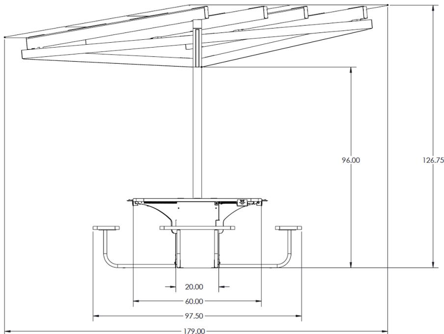
Note: Solar array has a 5° tilt
